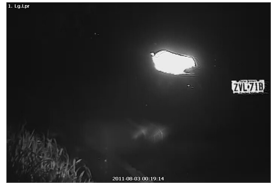
Actual Recorded Video Image of License Plate Capture Camera at Night on a Vehicle Traveling Approximately 45MPH
