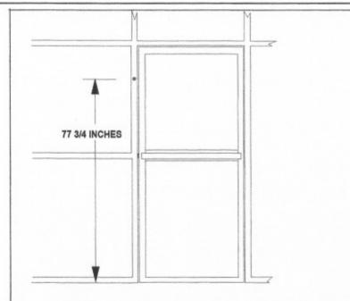
Drill feed-thru hole for cable on mounting surface 77 3/4" above the finished floor
