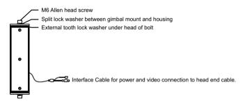
\* Camera lens position can be adjusted up and down 5 degrees
