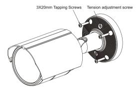
Position camera for best field of view then tighten camera/mount tension adjustment screws (x2)
