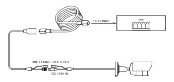
\* Diagram of typical modular wiring system connections
