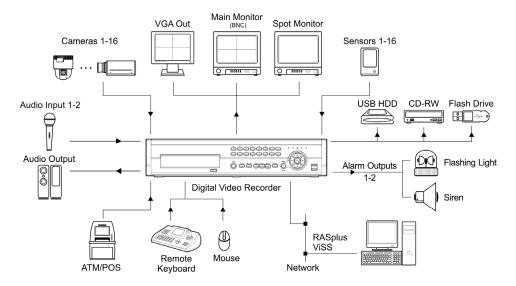
Figure 1 — Typical DVR installation.
