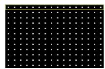
The Motion Detection Zone screen is laid over the video for the selected camera. You can set up motion detection zones by selecting or clearing blocks.
