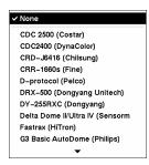
Select your camera from the list and press the button. You will need to connect the camera to the RS232 or RS485 connector on the back of the DVR following the camera manufacturer's instructions.
