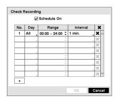
Highlighting Schedule On and pressing the button toggles On and Off. When set to On, you can select the day, time range and interval that you want the DVR to run self-diagnostics on the recorder. The Interval can be selectable from 1 min. to 7 days or Never. The box allows you to delete a check recording schedule.
